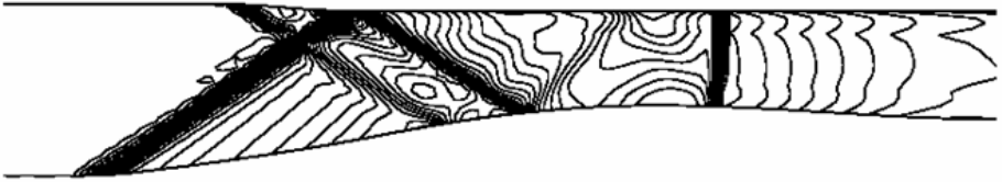
Figure 2. Contours of Mach number for steady flow through supersonic diffuser. Steady-state inflow Mach number is 2.2.
