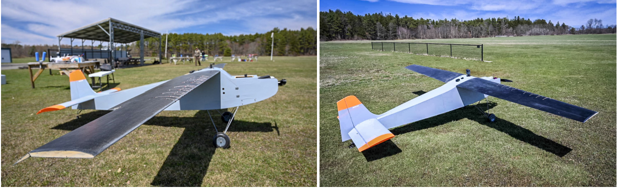
Fig. 3 The custom-built hardware testbed used in this research. We create a digital twin of this 12-foot wingspan aircraft, and update the digital twin in response to online data from structural sensors on the aircraft wings.
