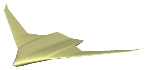
Figure 3: ESP representation of the BWB geometry.
