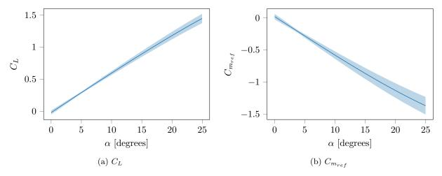
Figure 7: AVL aerodynamic coefficient estimates at Mach 0.3 with  $\pm 3\sigma_t$  confidence bounds with no control surface deflections.
