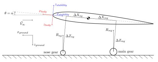
Figure 6: Axis systems for the BWB on the ground along with the gear reaction forces  $R_{mq}$  and  $R_{nq}$ .
