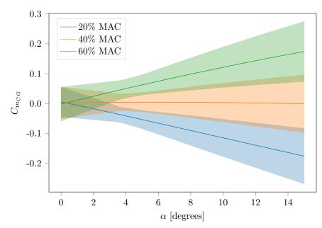
Figure 8: Estimates of the pitching moment about the center of gravity computed using Eq. 25 and the aerodynamic coefficients in Figure 7. The shaded areas represent the  $\pm 3\sigma_t$  confidence bounds.
